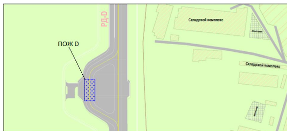
Figure L.1.7. Layout scheme of AIF-5 pad (PLs "V" and "T") for AC D/A with engines running in the area of RWY-3
